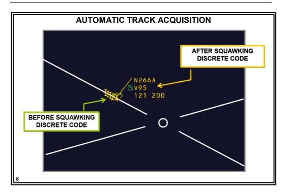
The full data block is automatically associated with the target symbol of an aircraft that is squawking a discrete code assigned by the computer.
